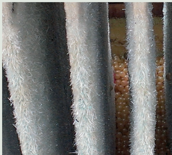
Figure 4: Gypsum formation on the lead anodes – the needle like crystal structure of selenite.
